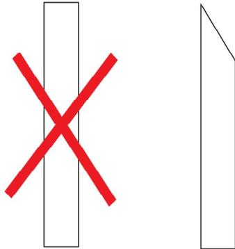
*It's important that the tip of the capillary is sharp to simplify the injection.*
