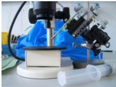
*The angle of the needle is approximately 60 degree, pressure is controlled by a 12 or 50 ml syringe.*
